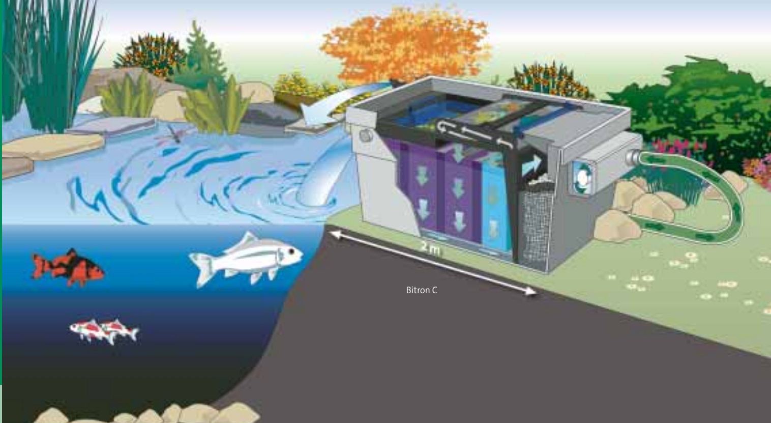
Schematic diagram: UVC clarifier in combination with OASE BioTec ScreenMatic 2 flow-through filter
