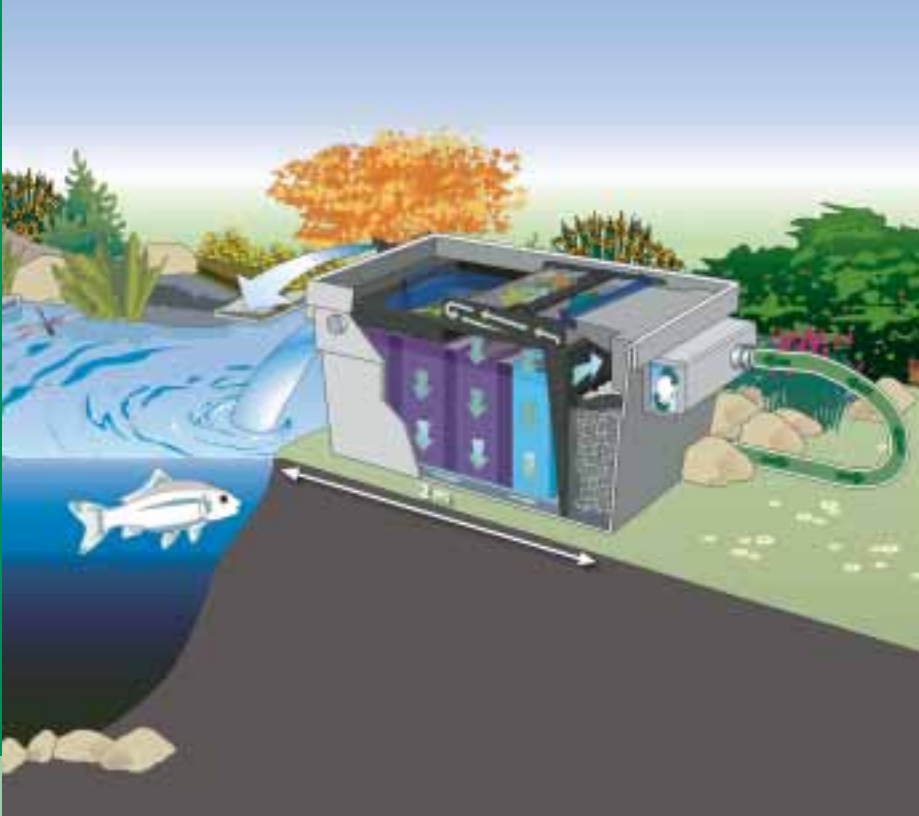
Schematic diagram: in combination with OASE BioTec ScreenMatic®
