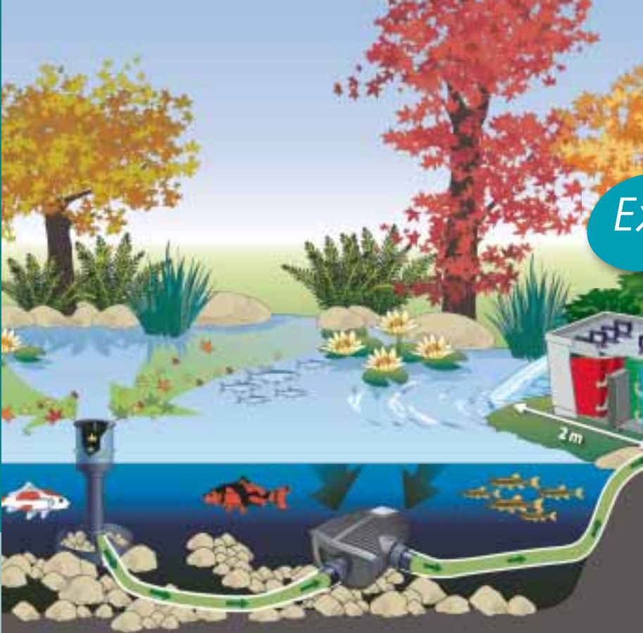
Schematic diagram: AquaSkim in use with filter and watercourse pump AquaMax Eco Premium
